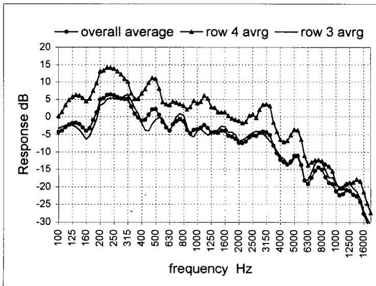
Fig. 15. Average of measured frequency responses of pelmet loudspeaker.
