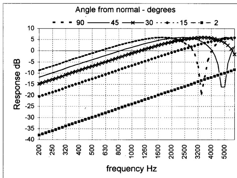
Fig. 3. Frequency response of ideal dipole with 100-mm spacing between drivers.
