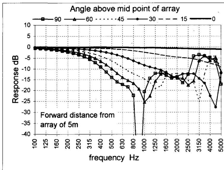
Fig. 19. Calculated frequency response above short line array.
