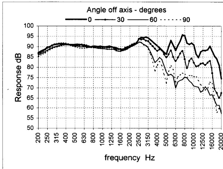
Fig. 2. Frequency responses on and off axis of Vifa S09FD driver at 1 W/1 m.
