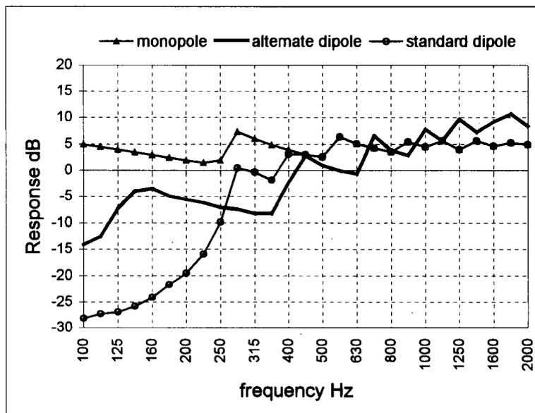
Fig. 6. Adjusted average frequency response of three systems in the tipstaves area.
