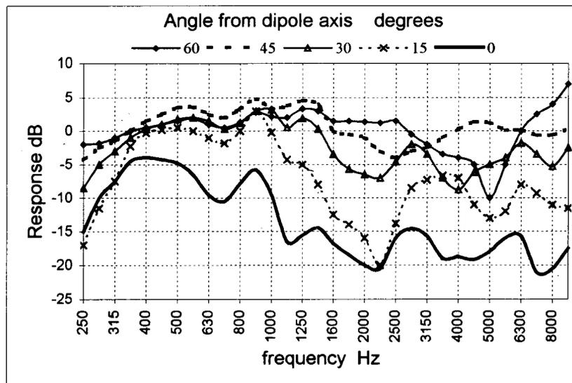
Fig. 9. Frequency responses of dipole in trough with reflector plates.
