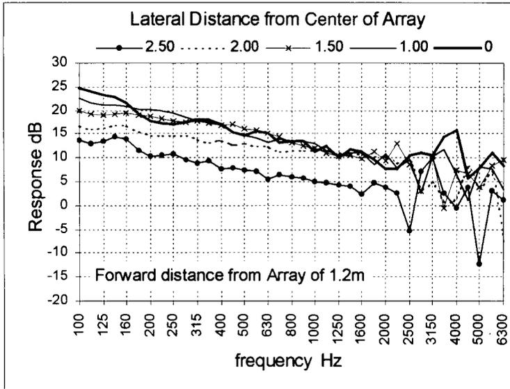
Fig. 13. Response along one-half of third seating row with acoustically curved array of 34 drivers on wall.
