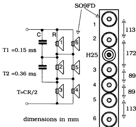
Fig. 18. Arrangement of drivers and tapering filter for short line array.
