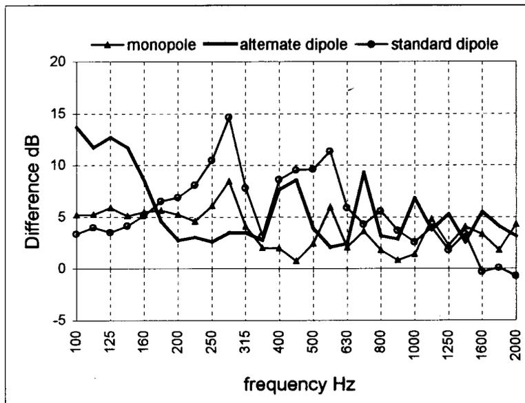
Fig. 4. Difference at each frequency between adjusted average level in tipstaves area and maximum level in microphone area.
