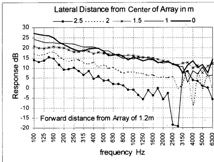
Fig. 12. Response along one-half of third seating row with flat array of 34 drivers on wall.
