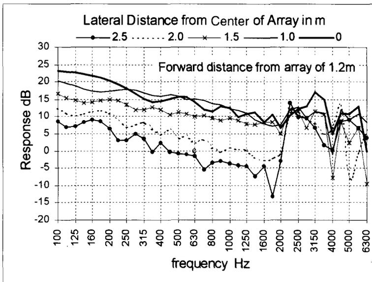
Fig. 11. Response along one-half of third seating row with array of 20 drivers on wall.
