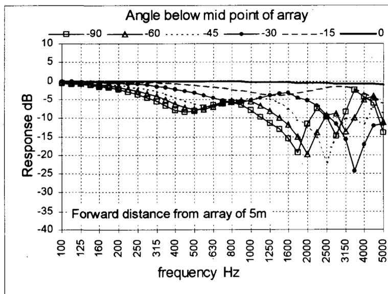
Fig. 20. Calculated frequency response below short line array.
