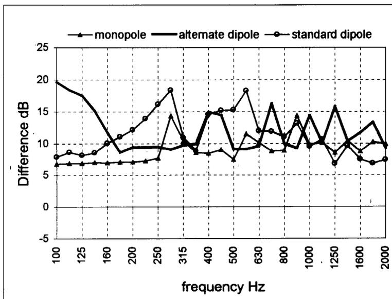
Fig. 5. Difference at each frequency between adjusted average level in tipstaves area and true average level in microphone area.
