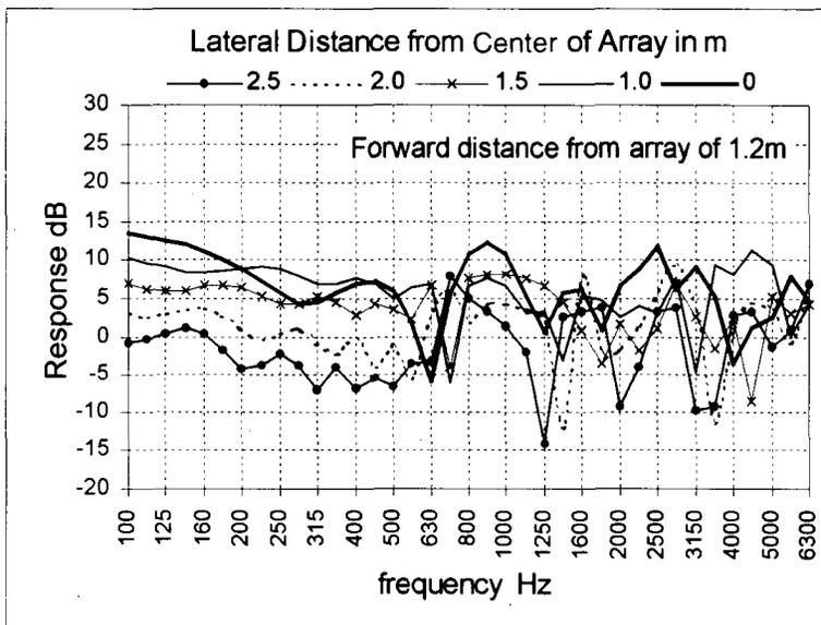
Fig. 10. Response across one-half of third seating row with array of 7 drivers on wall.
