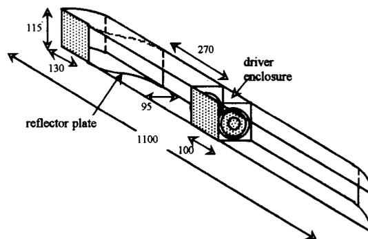
Fig. 7. Structure of dipole in trough. For clarity, reflector plate at one end is not shown.
