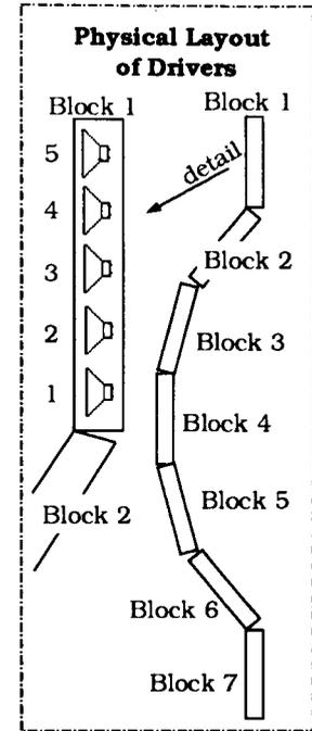
Fig. 16. Schematic diagram of pelmet array.
