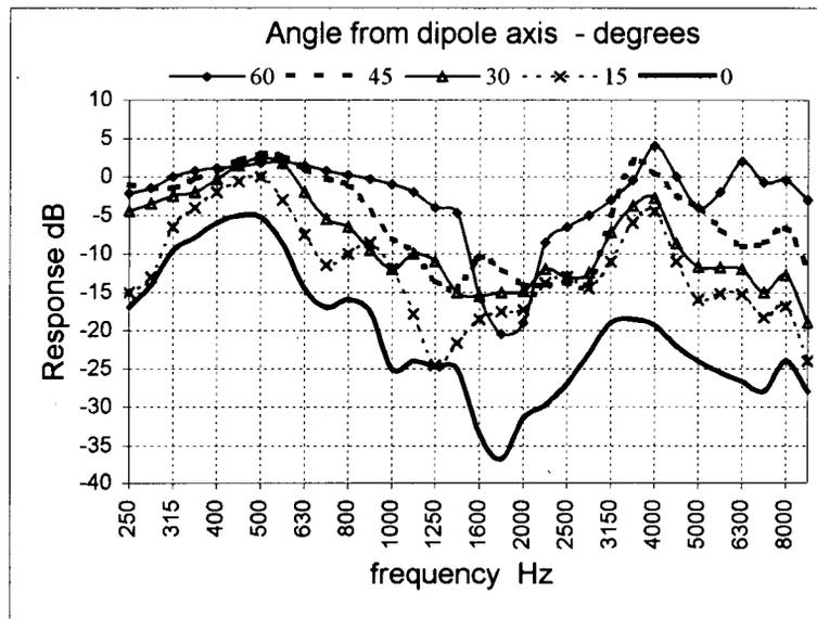
Fig. 8. Frequency responses of dipole in trough without reflector plates.
