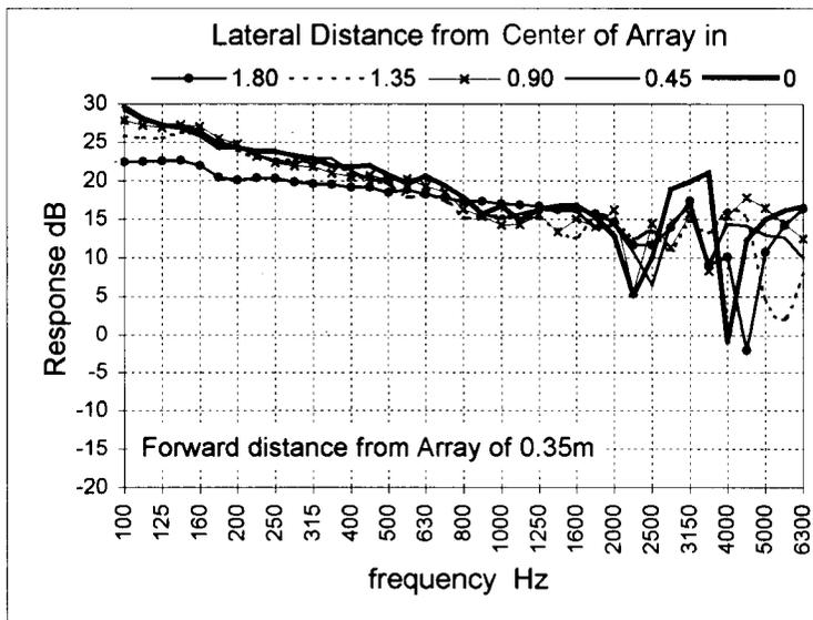
Fig. 14. Response along one-half of fourth seating row with acoustically curved array of 34 drivers.
