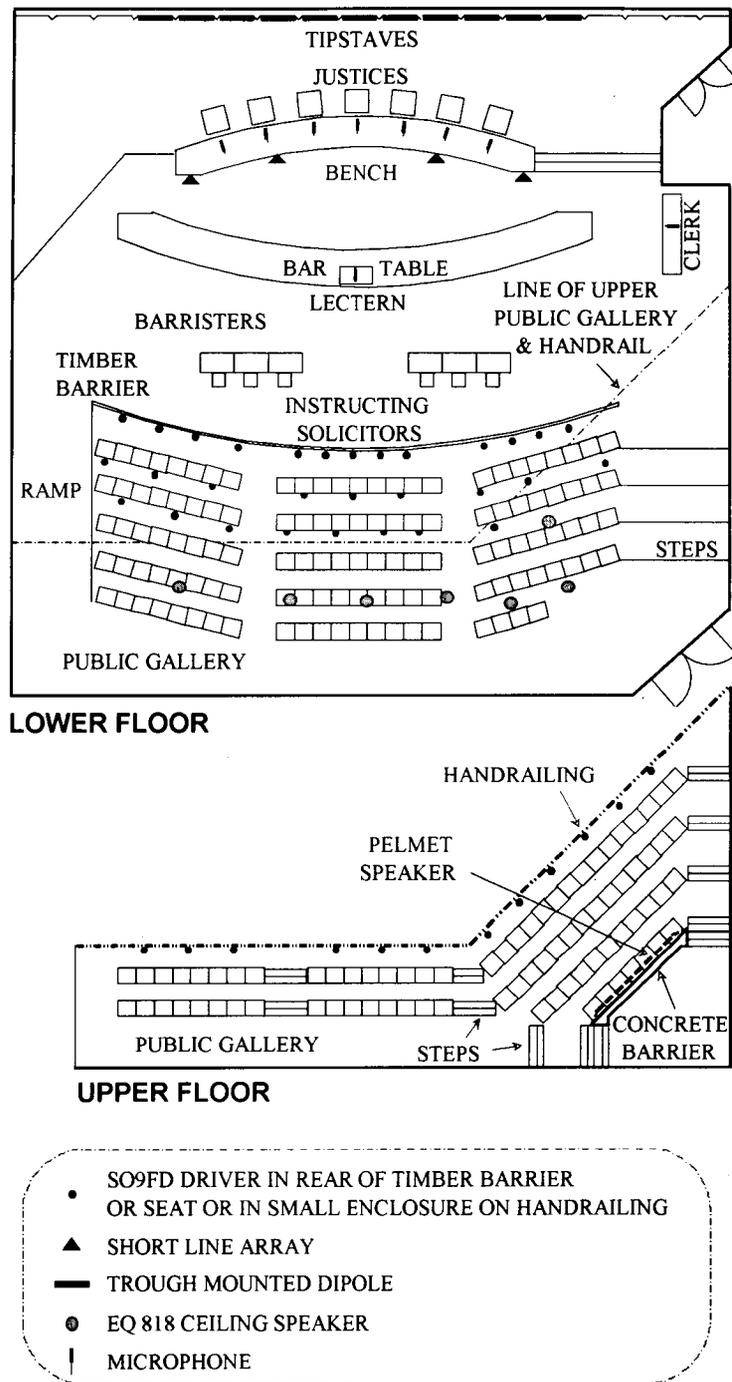
Fig. 1. Layout of room with locations of loudspeakers and microphones.
