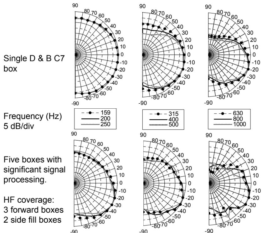
Fig.4 Comparison of polar responses for single C7 box with processed array of five C7 boxes
