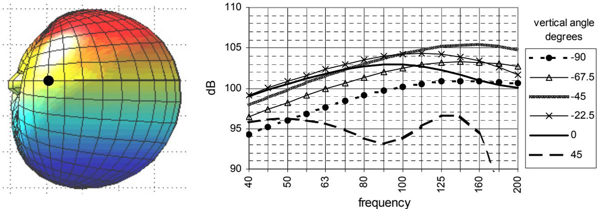
Fig. 14 Radiation balloon of subwoofer at 80 Hz
