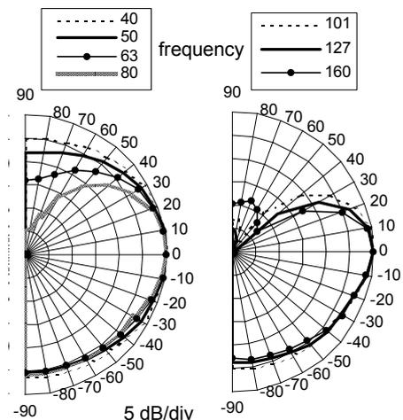
Fig.12 Predicted polar response of the subwoofer array
