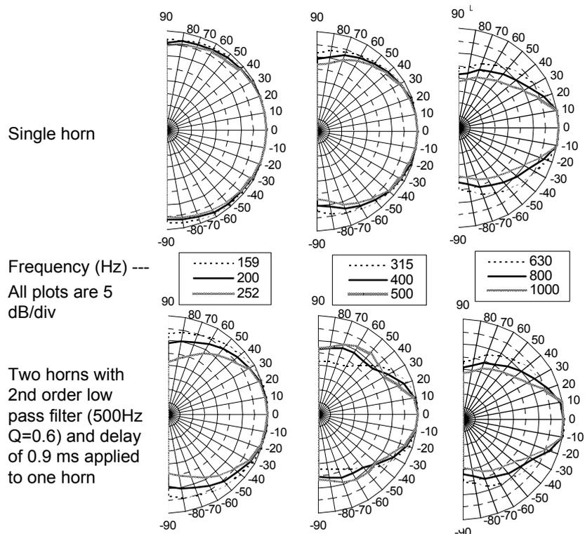
Fig. 5 Increasing the directionality of a 4402 mid-range horn
