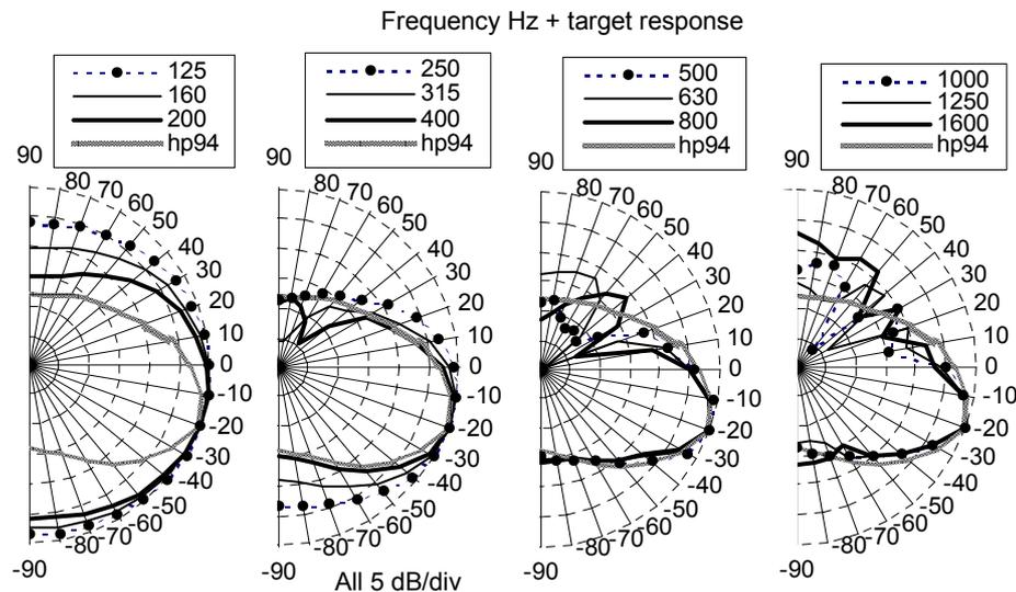
Fig. 7. Vertical polar response of gallery array
