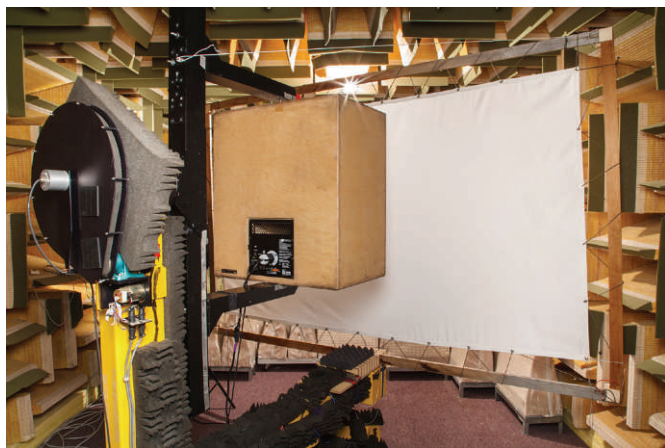
Figure 1. Speaker and screen with the positioning apparatus used in the anechoic chamber.
