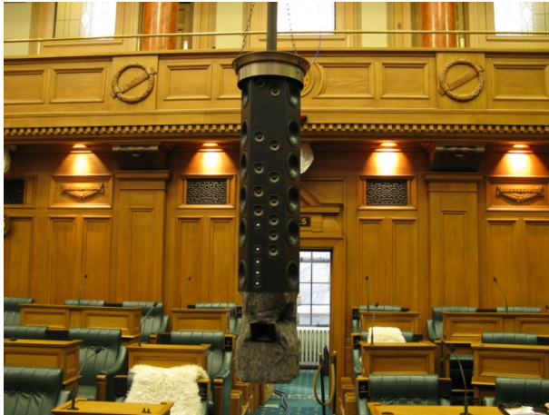
Figure 1: "Kiwi-tube" Multi-channel cluster of tapered arrays, horns and down-fill
