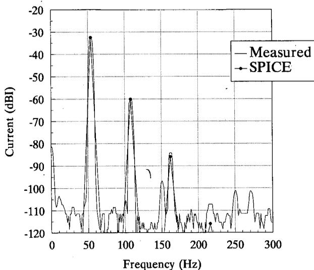
Fig. 9. Comparison of predicted and measured driver-current distortion at 54 Hz, -5 dBV input.
