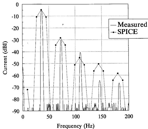
Fig. 8. Comparison of predicted and measured driver-current distortion at 36 Hz, +10 dBV input.
