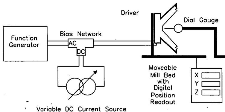
Fig. 3. Block diagram of equipment setup for measuring cone displacement against dc coil current.
