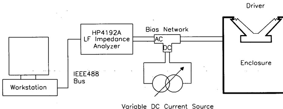
Fig. 2. Block diagram of equipment setup for measuring driver impedance for various dc coil currents.
