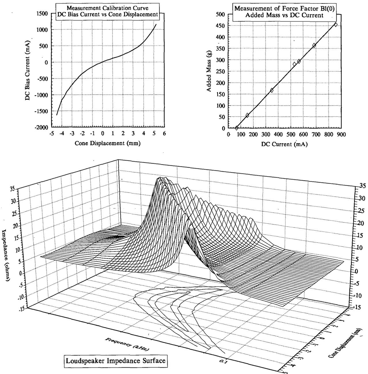
Fig. 4. Plot of data used for parameter extraction of Peerless 831921 driver. Impedance data were decimated for clarity.
