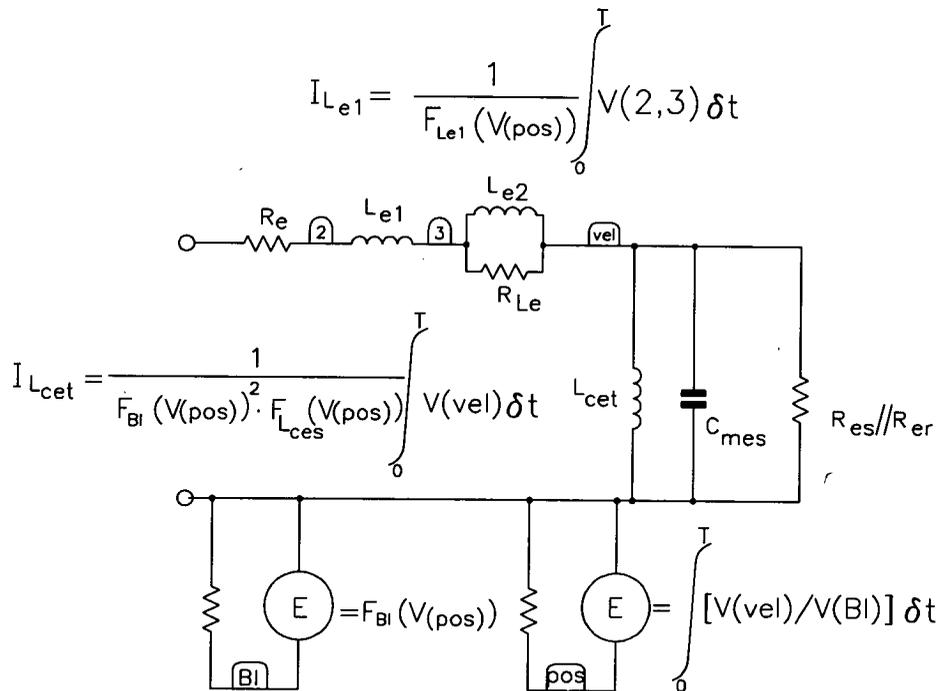
Fig. 6. Behavioral model of nonlinear driver as implemented in SPICE.
