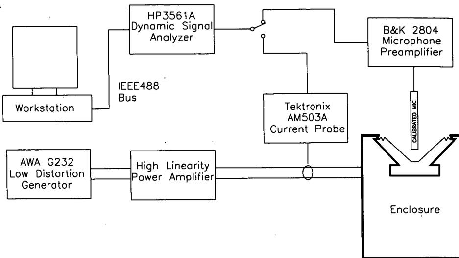
Fig. 7. Block diagram of equipment setup for measuring driver acoustic and current distortion.
