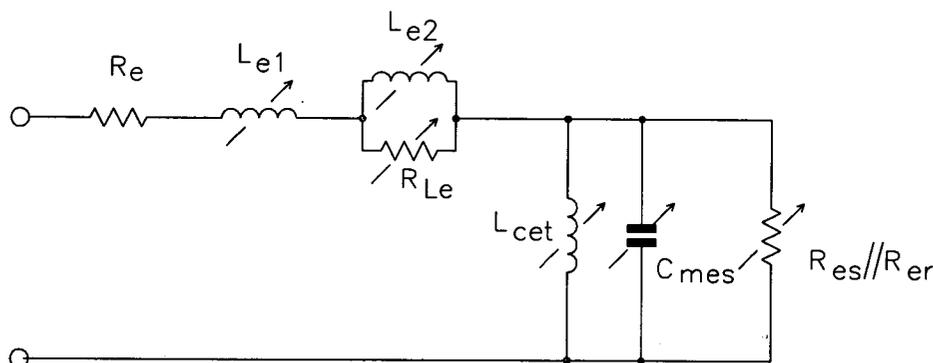
Fig. 1. Equivalent nonlinear circuit of driver.
