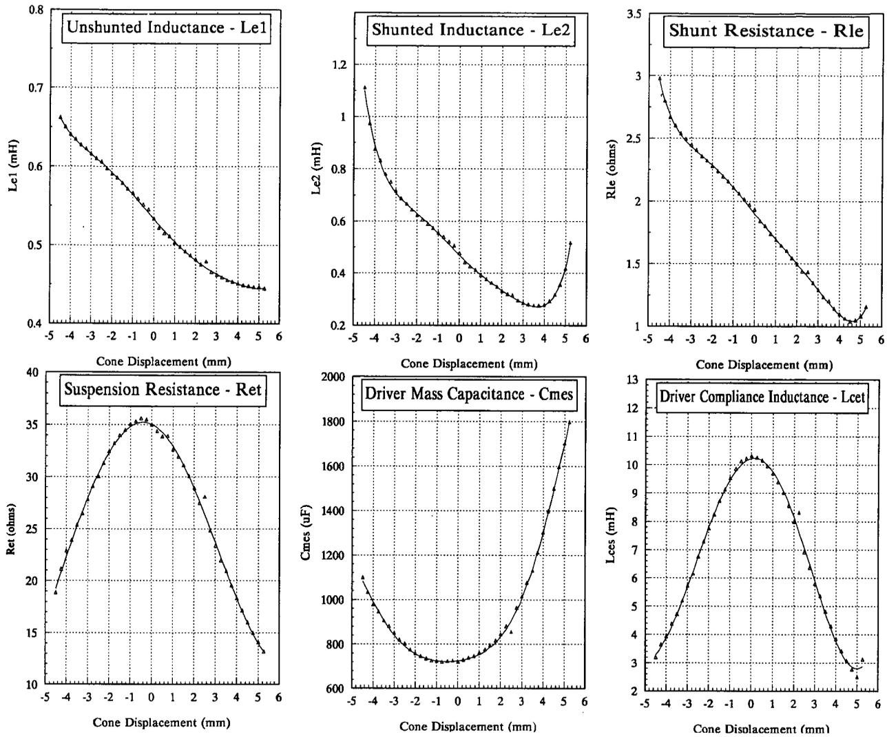
Fig. 5. Plots of nonlinear parameters extracted for 831921 driver.  $L_{e1}$ ,  $L_{e2}$ ,  $R_{Le}$ ,  $R_{et}$ ,  $C_{mes}$ , and  $L_{cet}$  versus cone displacement. Note that  $R_{et}$  and  $L_{cet}$  are box-modified equivalent parameters.
