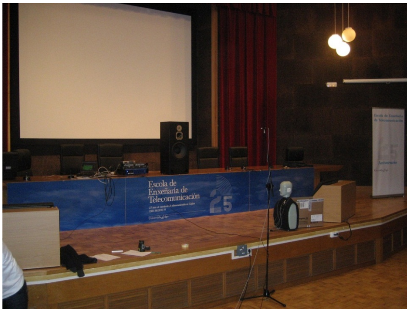
Figure 1 Loudspeaker in test auditorium as centre channel
