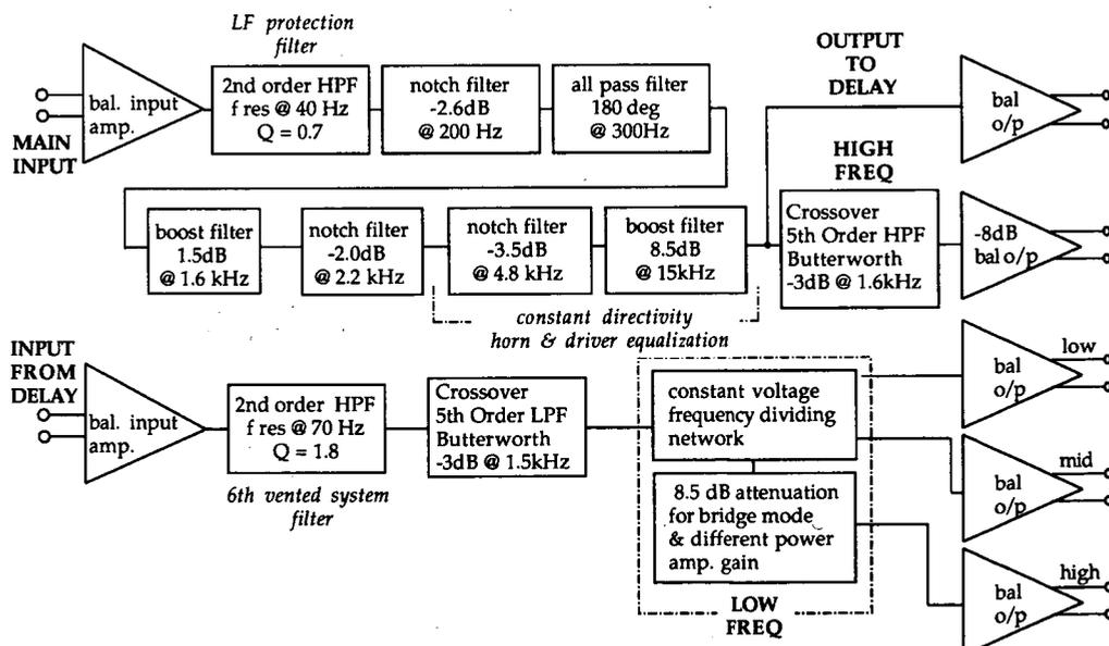
Fig. 7. Block diagram of type 1 signal processor.
