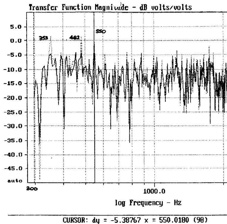
Fig. 13. Closed- and open-loop responses of loudspeaker-room-microphone system with 3-dB attenuation. -3 dB below regeneration—--- closed loop; ——— open loop.
