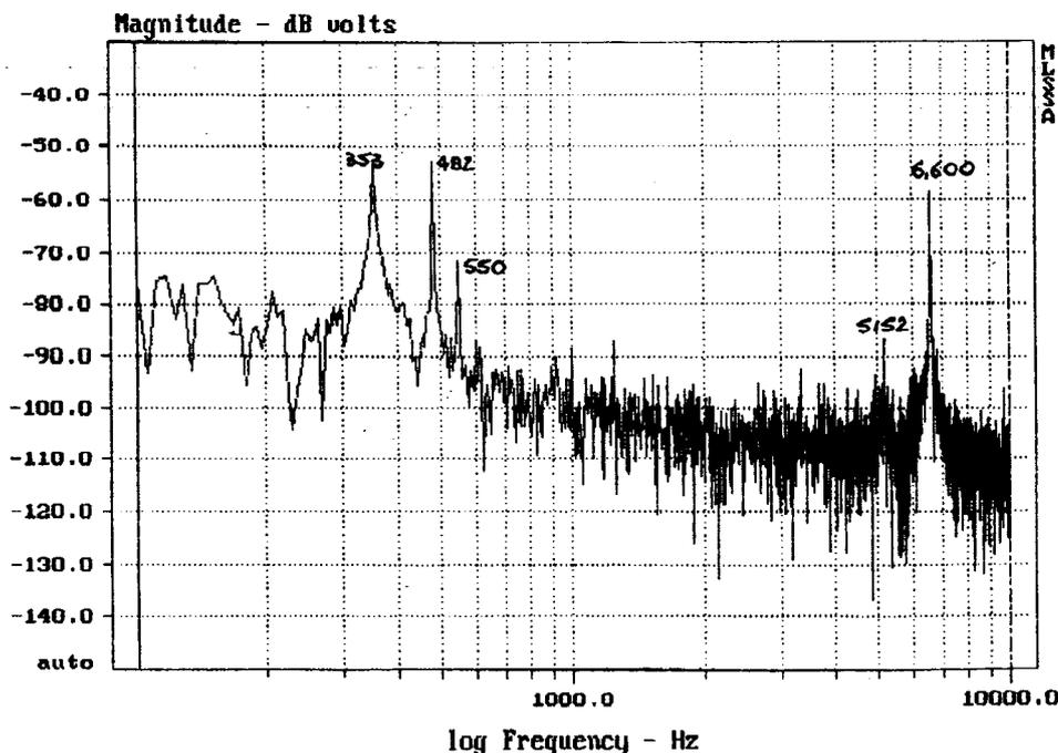
Fig. 12. Power spectrum of stable "ringing" feedback.
