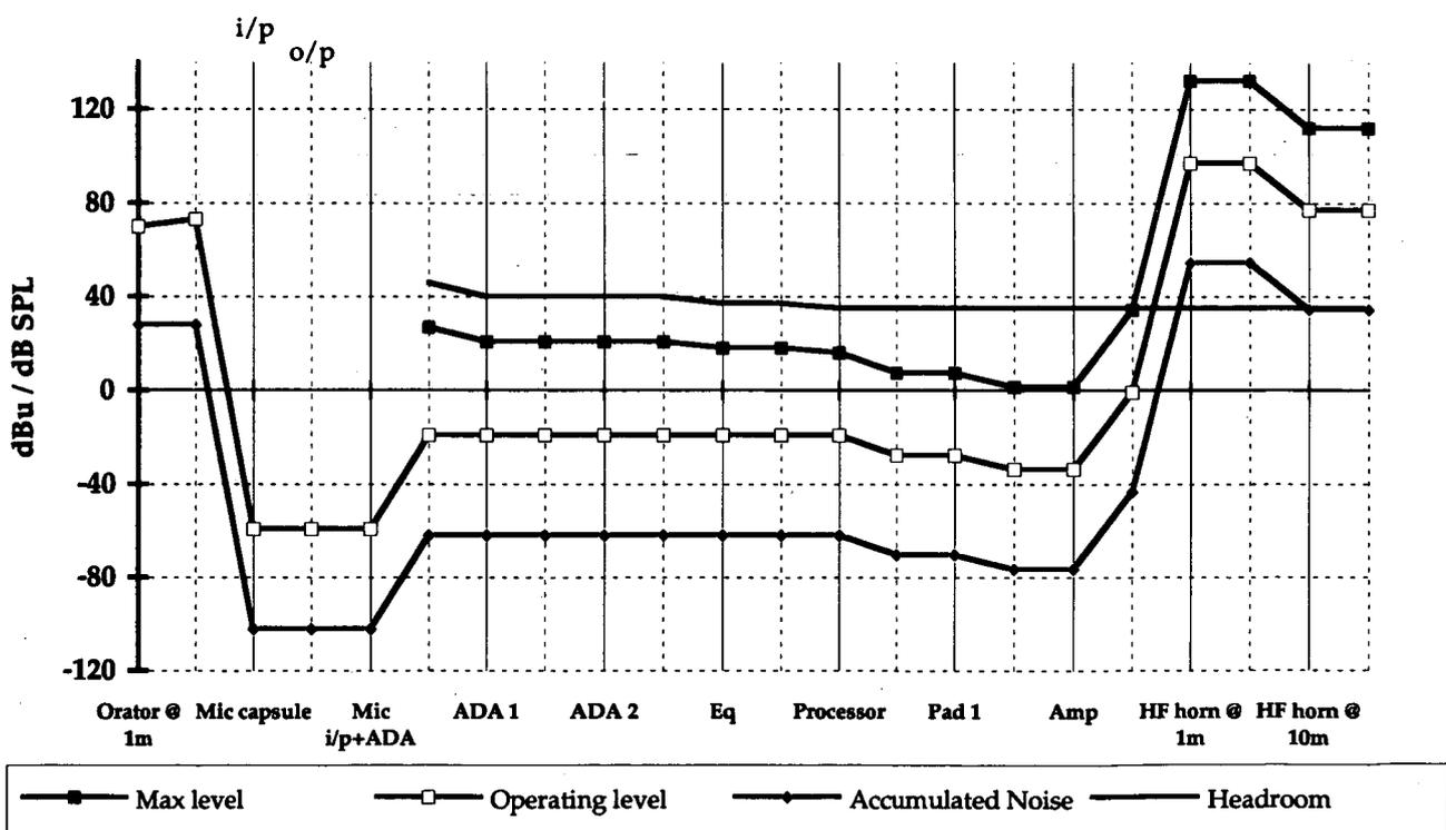
Fig. 9. Signal level diagram for high-frequency chain.
