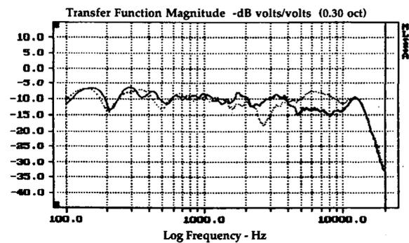
Fig. 8. 50-ms frequency response of prototype loudspeaker at two seating positions.
