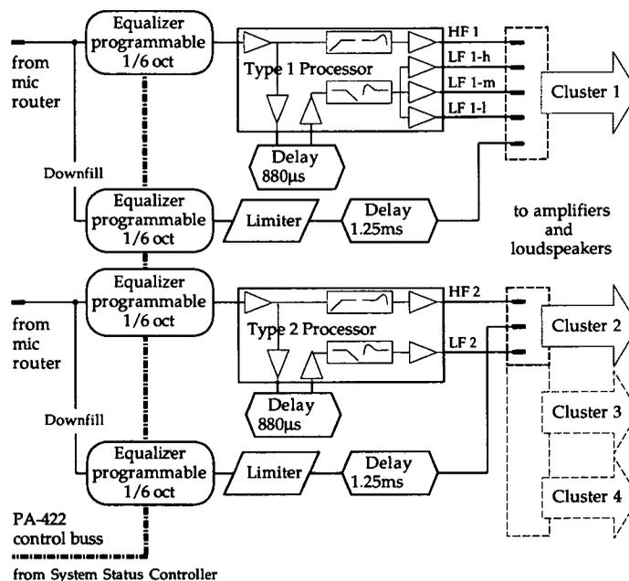
Fig. 6. Block diagram of signal-processing electronics.
