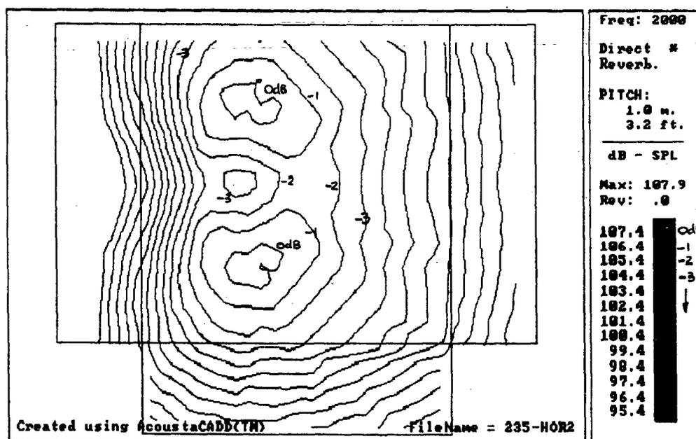
Fig. 3. Direct-field coverage pattern predicted by ACOUSTACADD.
