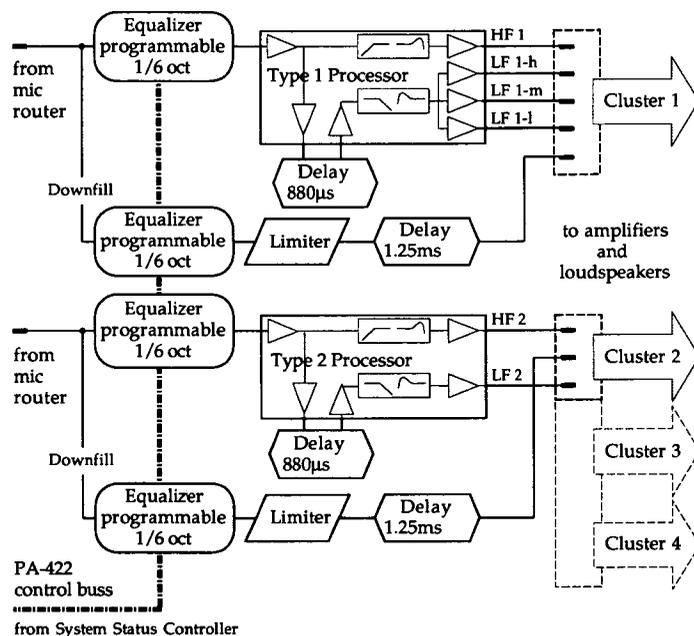
Fig. 6. Block diagram of signal-processing electronics.
