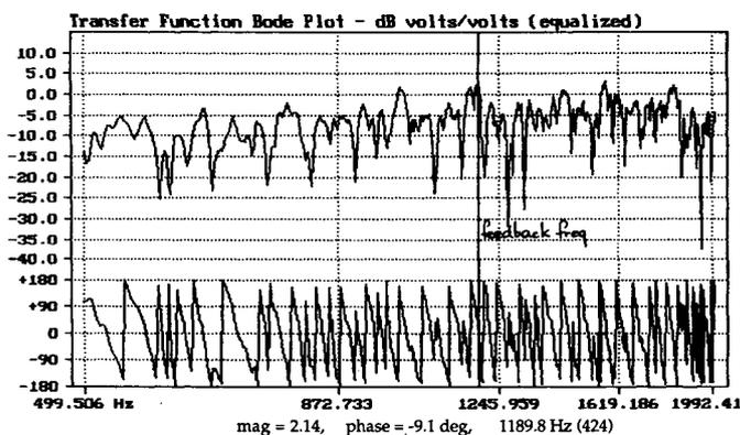
Fig. 11. Measured open-loop amplitude and phase response of loudspeaker-room-microphone system.
