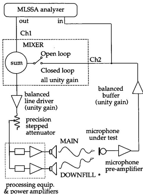
Fig. 10. Setup for measurement of system open- and closed-loop gain. \*Not used in laboratory setup.
