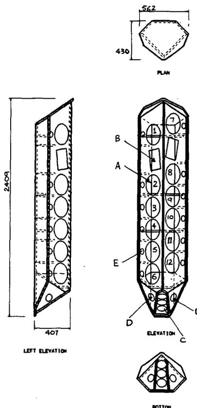
Fig. 2. Driver layout in loudspeaker enclosure. A—2123 drivers; B—HP94 horns; C—2105 drivers; D—2404 horn drivers; E—vents.
