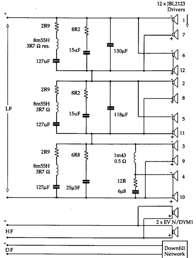
Fig. 5. Circuit diagram of type 2 passive filter network.
