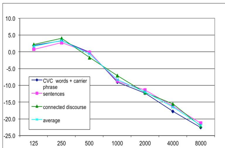
Figure 1 Speech spectra in dB relative to 0 dBA as a function of octave band frequency for TNO speech material.
