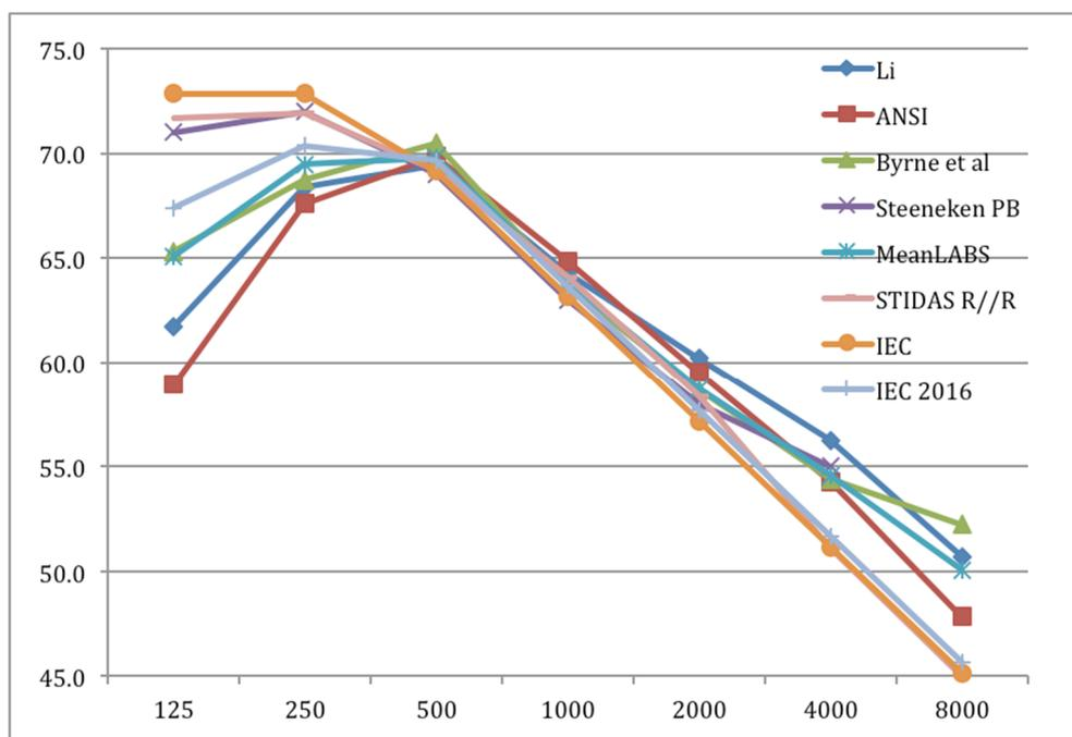
Figure 2 Speech spectra and STI test signal spectra from different laboratories in dB as a function of octave band frequency
