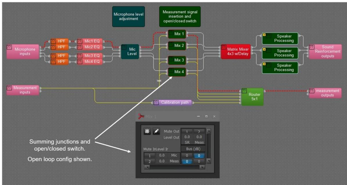
Figure 12 Block diagram of typical configuration of DSP unit for measuring loop gain.
