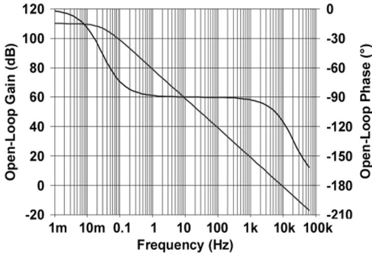
Figure 5 Typical open-loop gain and phase response of an op-amp
