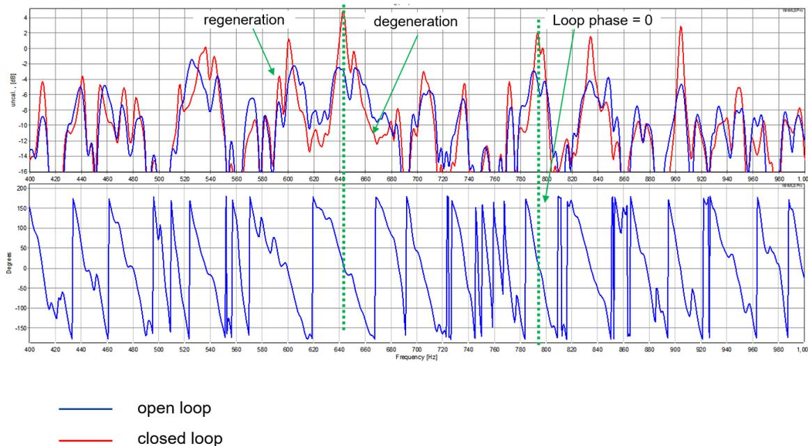
**Figure 8 Open and closed responses of a speech reinforcement system.**
