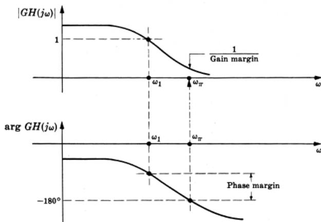
Figure 9 Generic open-loop gain showing amplitude and phase.
