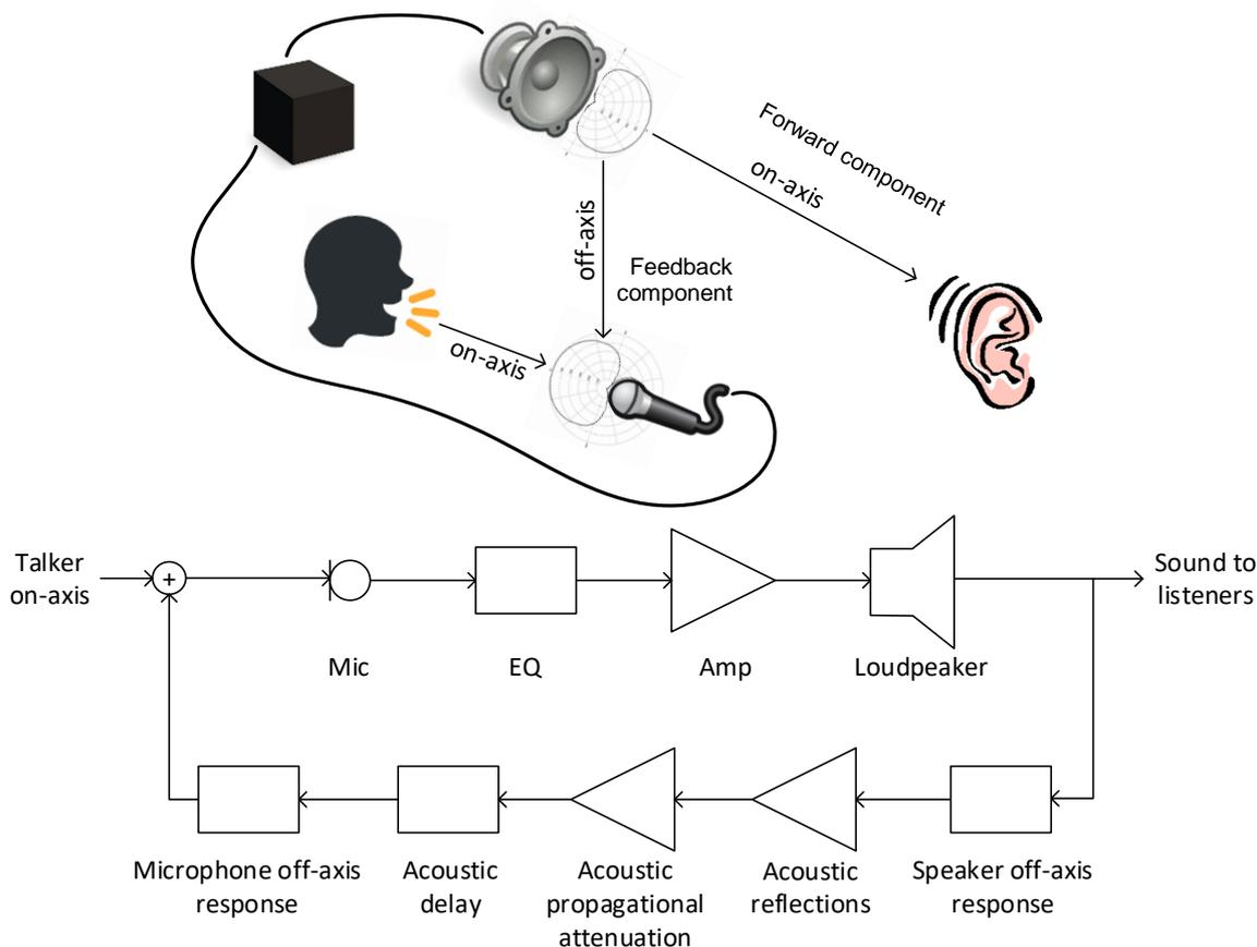
**Figure 4 Acoustic feedback loop system.**
