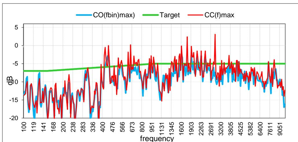
**Figure 11** Example of closed and open loop magnitude responses and the equalisation target.
