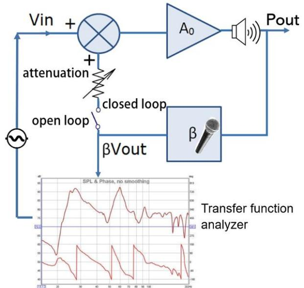
Figure 6 Schematic arrangement for measurement of open and closed loop responses of a sound system.
