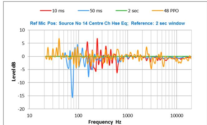
Figure 3 Responses shown in (4) with different windows at reference position of a Center Channel. NB 10 ms and 50 ms responses are truncated according to the time/frequency limit.
