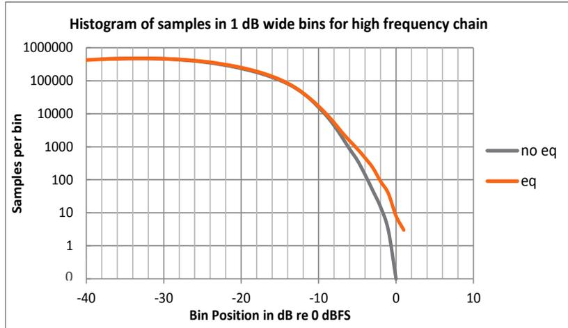
Figure 14 Histograms of signal levels in the high frequency chain with and without equalisation. Note the ordinate scale is logarithmic axis to allow comparisons at bin-position values close to 0 dBFS. (1200 Hz)
