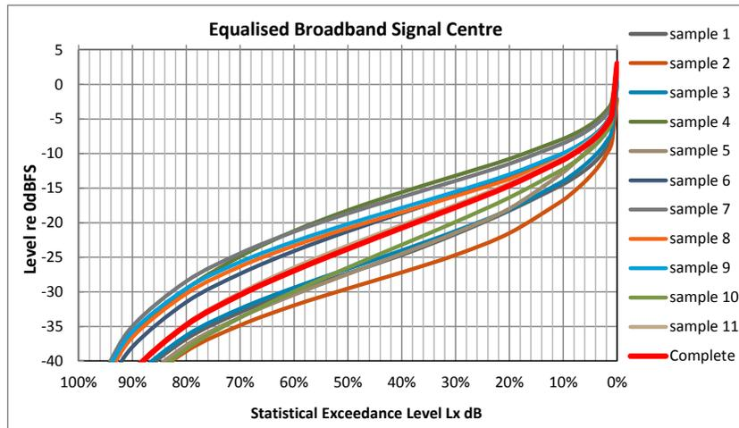
Figure 9 Exceedance values 0% to 100% for equalized broadband center channel signal ((1200 Hz crossover)
