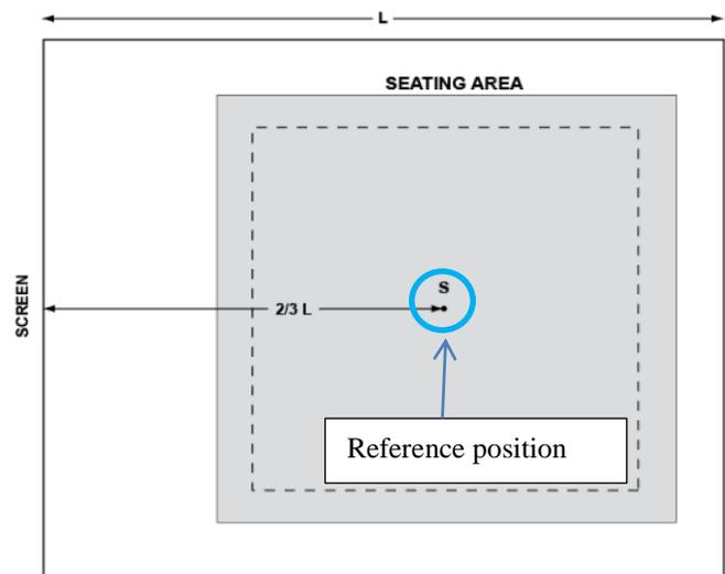
Figure 2 Physical layout of the reference position in a cinema.
