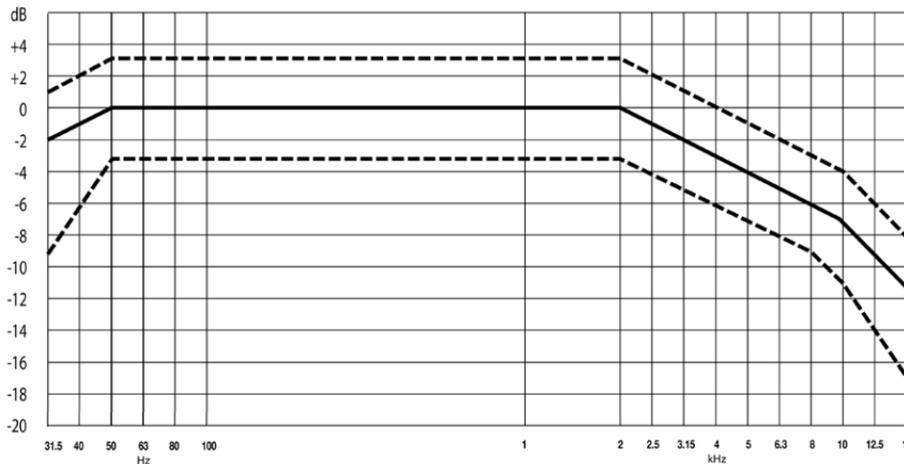
NOTE – Tolerances in this figure are based upon 1/3-octave measurements. If 1/1-octave measurements are used, reduce the tolerance by 1 dB.
