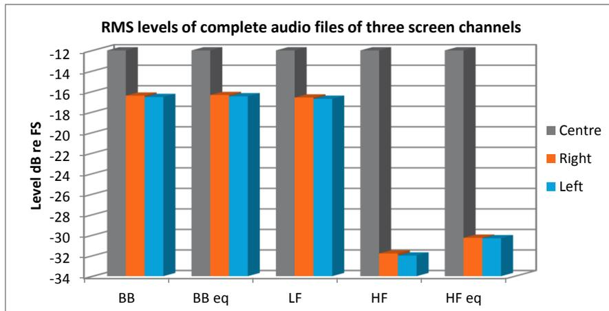
Figure 7 Computed RMS values for five signal chains of the three screen channels with 1200 Hz crossover.
