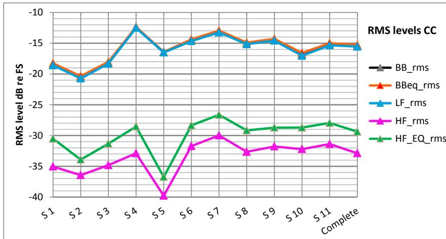
Figure 6 Computed RMS values for five signal chains of the Centre Channel with 2500 Hz crossover.
