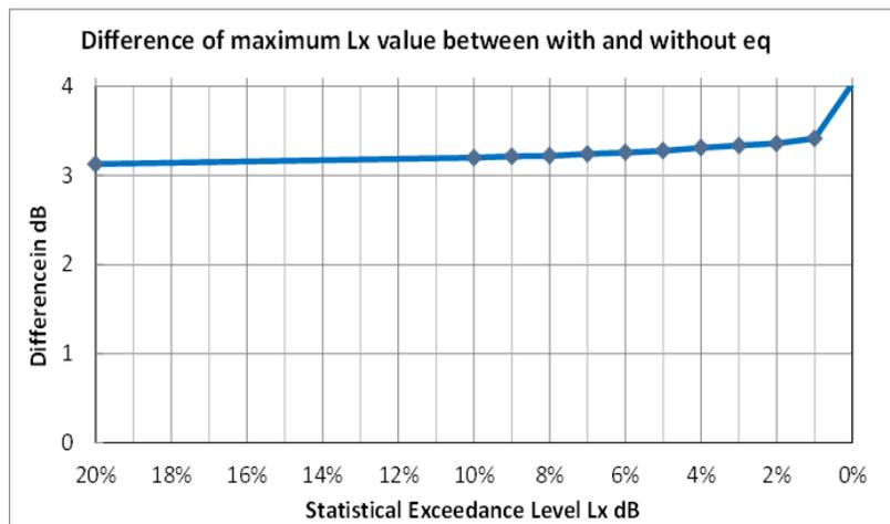
Figure 13 Difference of exceedance values for equalized and unequalized high frequency center channel chains with 2500 Hz crossover.
