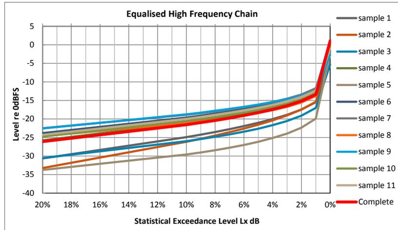
Figure 11 Exceedance values 0% to 20% for equalized high frequency center channel signal. (1200 Hz crossover)
