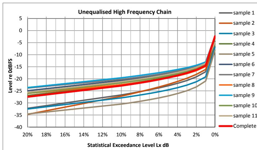
Figure 10 Exceedance values 0% to 20% for unequalized high frequency center channel signal. (1200 Hz crossover)
