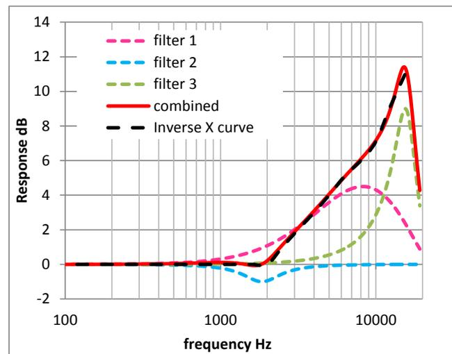
Figure 4 Responses of peaking IIR filters and inverse X curve.
