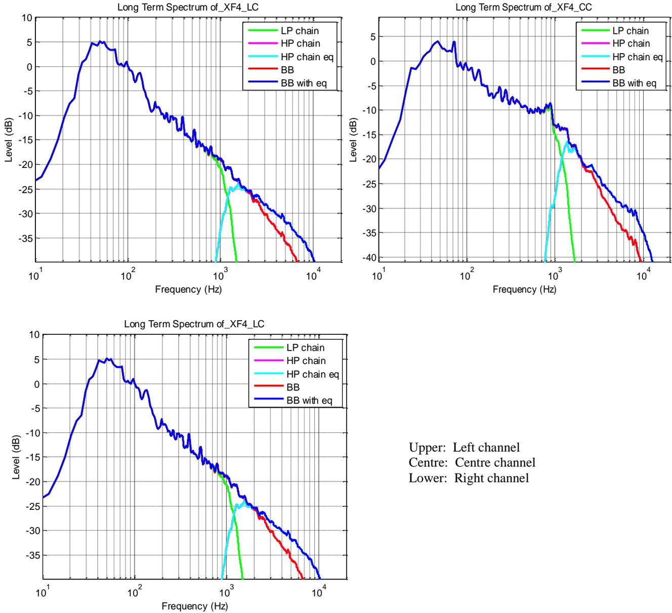
Figure 15 Power Spectral Density of the five signal chains of the three screen channels. 1200 Hz crossover system shown.
