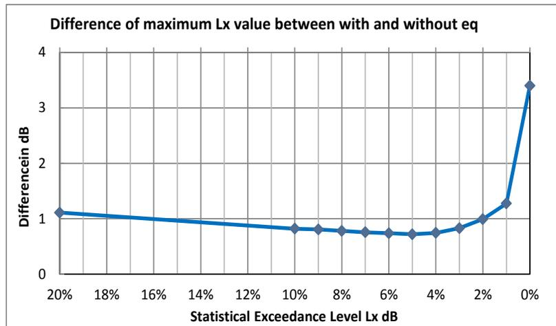
Figure 12 Difference of exceedance values for equalized and unequalized high frequency center channel chains with 1200 Hz crossover.
