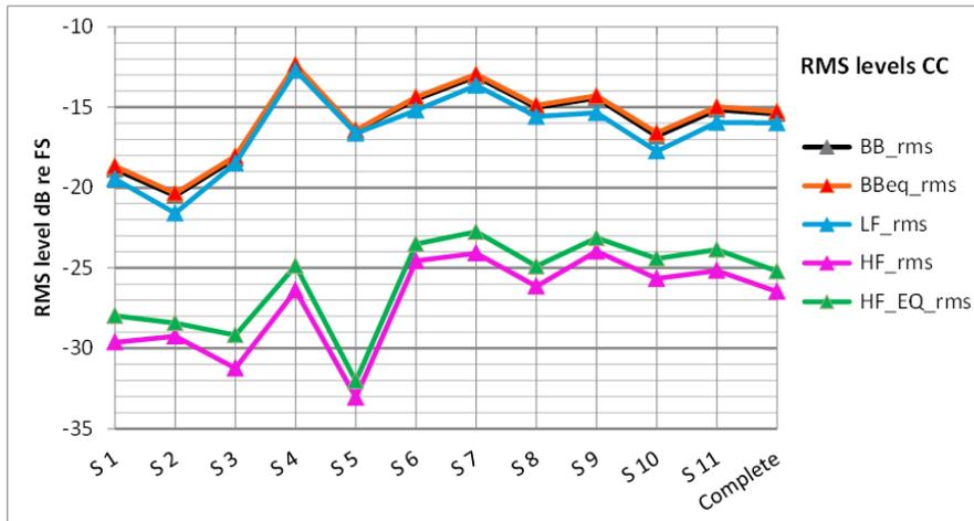
Figure 5 Computed RMS values for five signal chains of the Centre Channel with 1200 Hz crossover.
