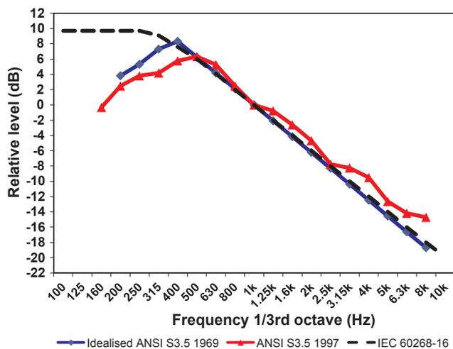
Fig. 1. Male speech spectra from different sources. All the spectra levels are normalised to 0 dB at 1 kHz.
