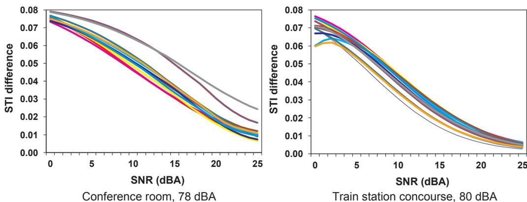
Fig. 9. STI difference between the use of the IEC spectrum and the proposed male spectrum, against the average SNR (dBA). STI calculations are presented for each of the 12 positions.
