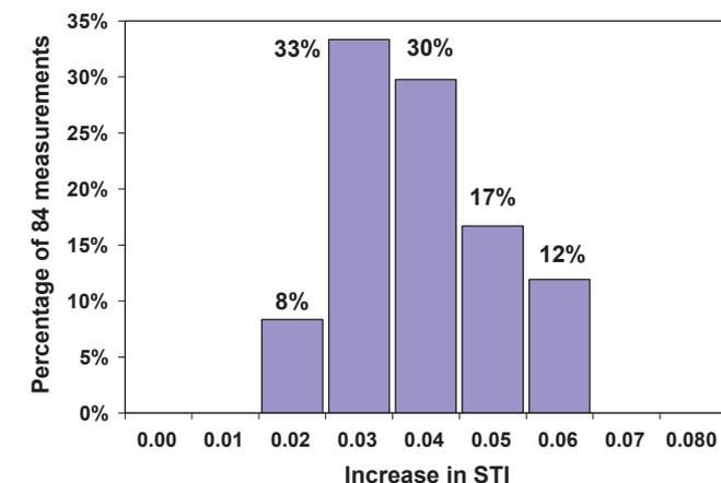
**Fig. 8.** Percentage distribution of the increase in STI obtained with the proposed male spectrum for a total of 84 positions taken over the voice alarm systems.
