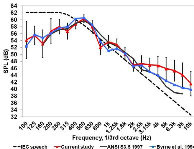
Fig. 4. LTASS for this study measured at 0.5 m with Harvard sentences and other spectra. Error bars indicate one standard deviation. All spectra were normalised to an overall level of 64 dBA.
