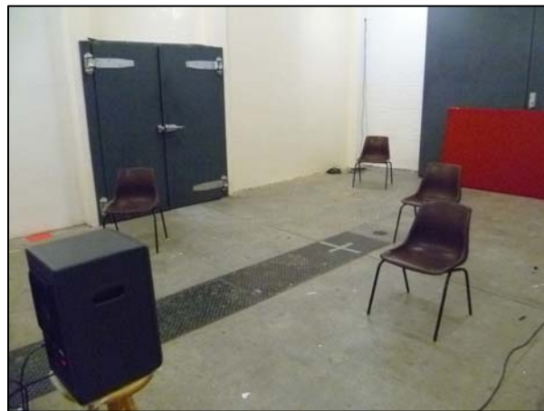
Figure 1. Reverberant chamber in one of the reverberation scenarios. A few of the listening positions and the monitor loudspeaker used for the listening tests are shown.
