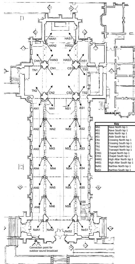
Some 44 Acoustic Technologies ALA07C arrays were carefully positioned on columns throughout the cathedral.
