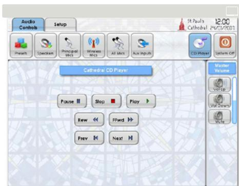
The AMX system control provides easy access to a selection of presets, as well as the ability to turn on/off microphones, speakers, playback and additional auxiliary inputs.
